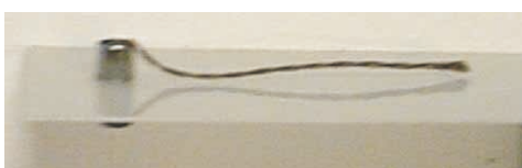
Nylon wiper with pre-assembled shunted brush
